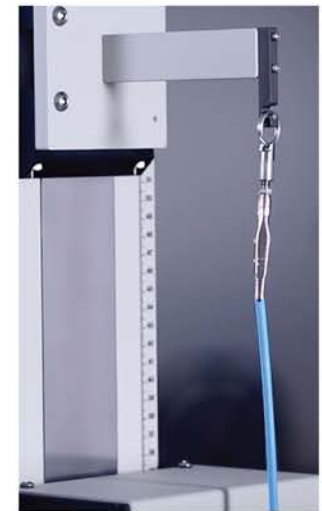
Accommodates parts from 0.3 mm - 20 mm in diameter, with lengths up to 70 cm
